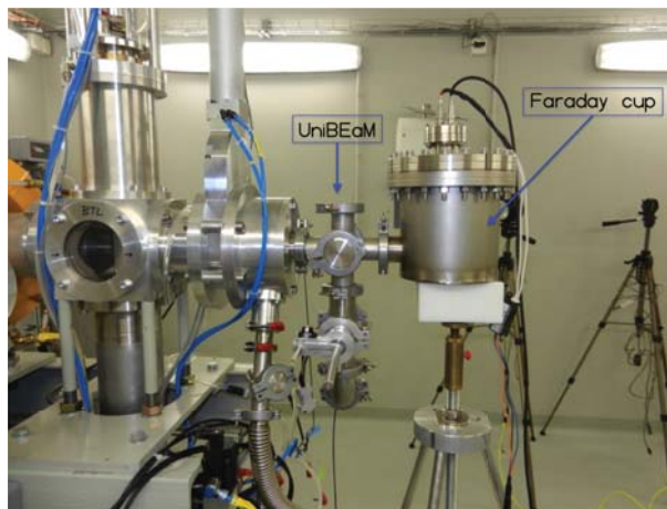
Fig. 7. Faraday cup installed on the BTL.
