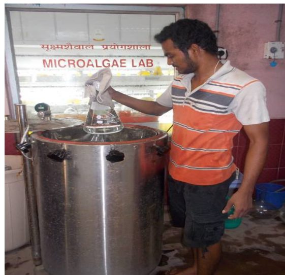
Fig. 2 Heat sterilization by autoclaving
