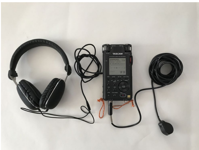
FIGURE 2 Typical recording equipment for PASS, consisting of headphones, recording unit, and cabled hydrophone
