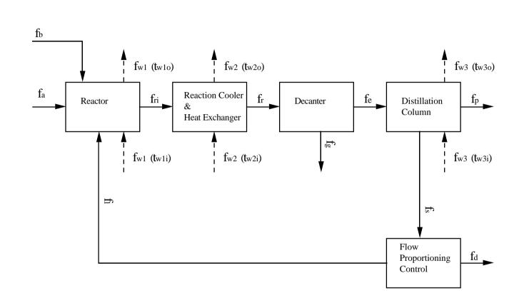
Figure 1. A Generalised Chemical Process Model for Control
