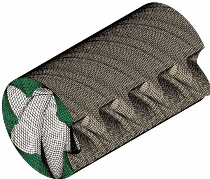
Figure 1 Configuration of a structured numerical mesh for the flow domain of the male rotor
