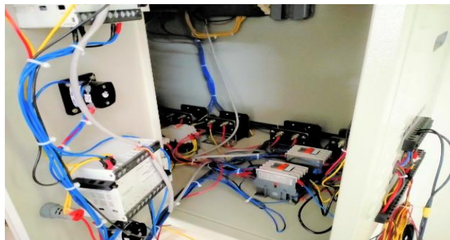
FIGURE 16. RS485 for communication system
