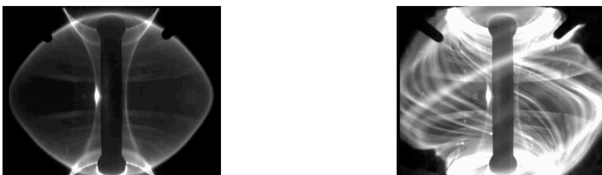
Figure 1. (left) A tokamak plasma in high-confinement mode (or “H-mode”) has a well-defined edge and good confinement of heat; (right) but these plasmas suffer from edge-localised modes (ELMs), which last only about 100\mu\text{s} yet during which over 10% of the total stored energy may be lost. (Images from the MAST tokamak.)
