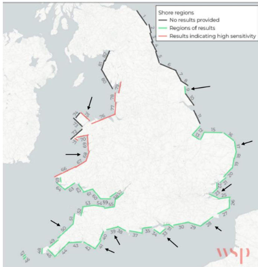
Figure 1.- Model regions; note that (1) black lines indicate regions where results could not be calculated, due to issues with the representation of Holocene sea levels, (2) red lines show areas of particularly high sensitivity and (3) Regions 14, 24 and 56 are not labelled, but exist in (clockwise) sequence. Black arrows indicate the regions on which the study cases have been selected (source “the User Guide” [1]).
