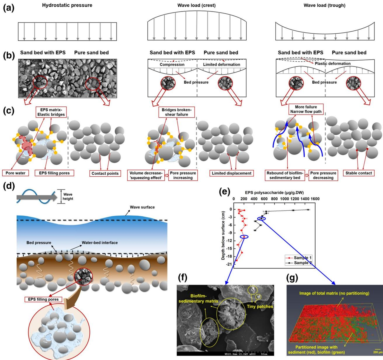
Note: the “compression” or “deformation” of the bed only represents a “tendency” before the liquefaction occurs, after which a fluid-like motion of the bed can be observed, and the sediment-water interface oscillates.
