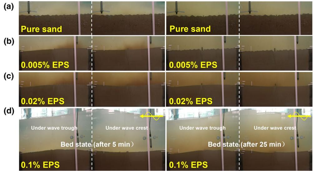
**Figure 1.** Photographs of bed state during tests. (a) Test 1 (0% EPS), (b) Test 2 (0.005%), (c) Test 4 (0.02%), and (d) Test 6 (0.1%), looking in the side view of the flume and perpendicular to the direction of wave progression. Two bed states under a wave trough are given after 5 min (left column) and 25 min of wave action (right column). The length of the pit is 1 m. EPS, extracellular polymeric substances.
