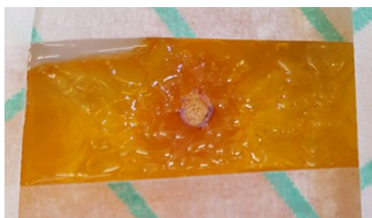
Figure 6.19 He-CAP treated ARS-PBA hydrogel. Edges of the gel were taped down to prevent movement.
