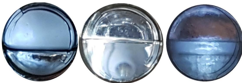
Figure 5.32: Images taken at 50 bar (left), 90 bar (centre) at 50 °C with a 4 mol% mixture of DMC and water in methanol. Right image at 70 bar CO 2 , 50 °C with a 7 mol% mixture of DMC and water in methanol.
