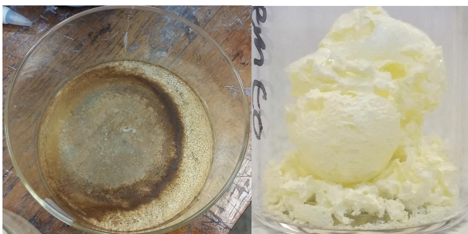
Figure 2.2: Left: Cerium nitrate precursor after the pre-treatment step at 150 °C. Right: Final calcined cerium oxide.
