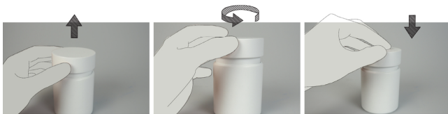
Figure 5: The embodied password interface. To start the password you lift the top part, after which you can start rotating. In order to enter the password, the top part is pushed back in.
