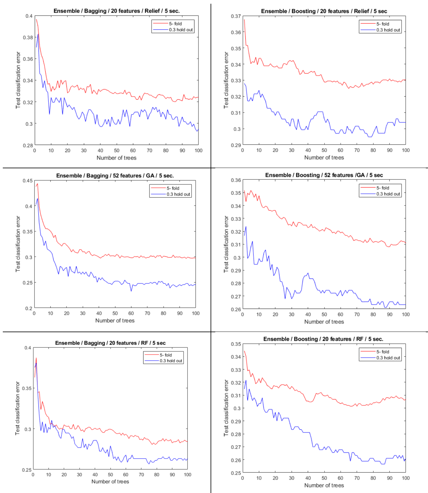
Appendix H. 3 Validation techniques comparison (5-fold & 0.3 hold-out) of Ensemble classifiers (Bag & Boost) for DataSet1_all (3 FS: ReliefF, GA, RF), FOSW segmentation method over 5 sec. window .
