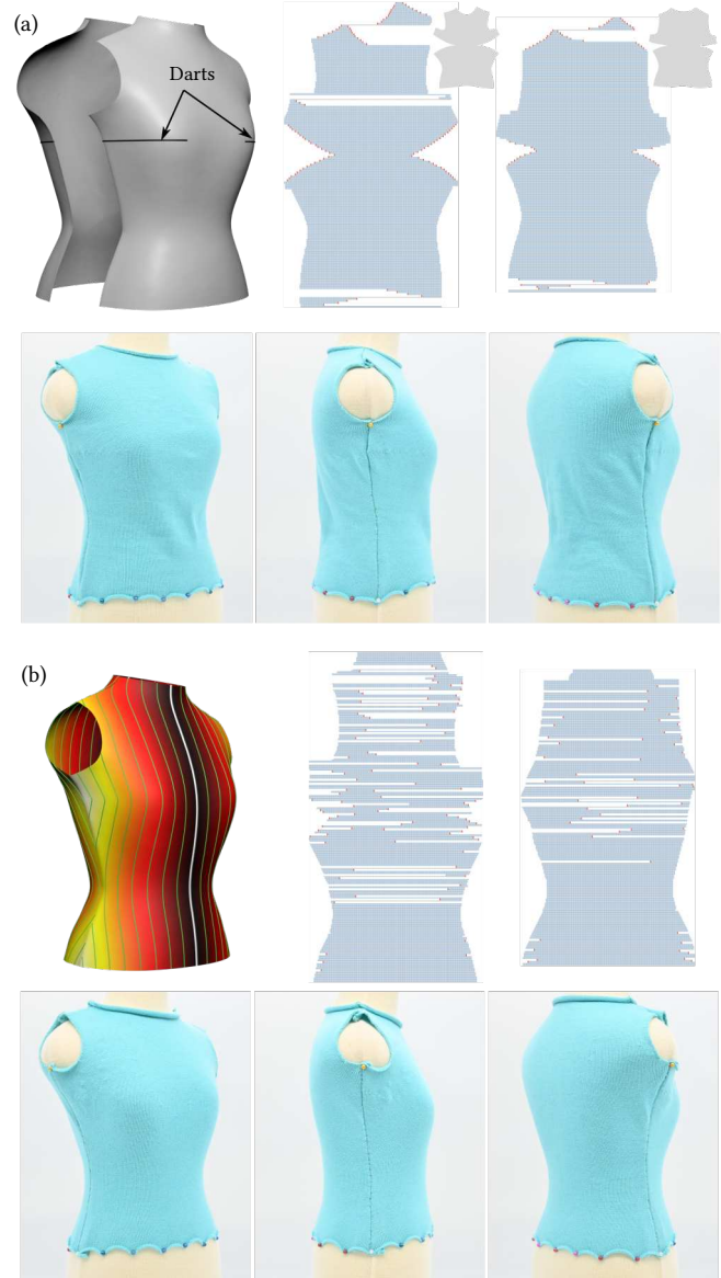
Fig. 12. Comparison of knitting maps generated from the flattened 2D panels with manually added darts (a) vs. from the 3D surface with the help of geodesic distance-field (b). The same set of pin holds are used for the two tests. The physical knitting results show the advantage of our approach with improved fit of the final garment. Note that the 2D panel results are generated by [Liu et al. 2008] without applying any scaling. Although scaling down the 2D panels can improve the fit at the waist, it will also make other parts of the garment too tight.
