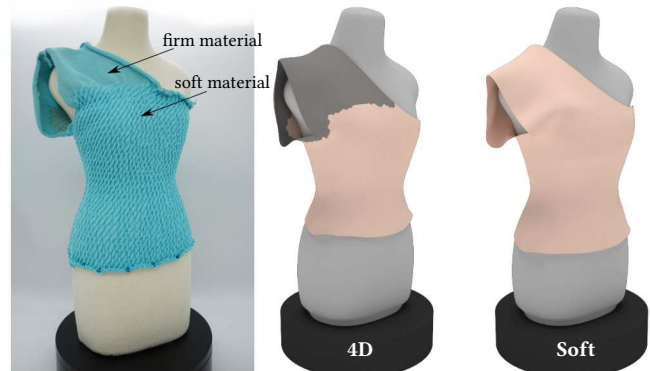
Fig. 17. One-shoulder knitted top with prescribed material distribution to achieve a desired shape. Firm material on the shoulder produces a stiff style, while soft material on the torso ensures comfort. From the simulation, it can be found that the style cannot be achieved using a uniformly soft material.
