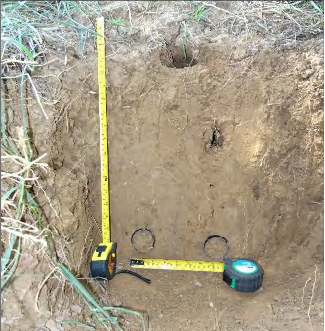
Figure 5. Sampling location ÇHI7A3 showing the location of the two sampling tubes inserted into the profile to collect undisturbed material for OSL dating.
