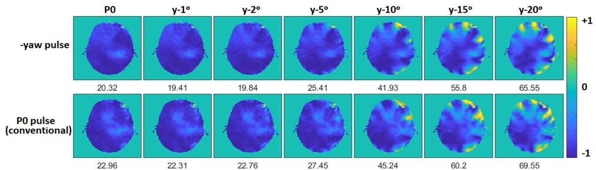
**Figure 3.** Inversion profiles at slice 2 following in-plane rotation (-yaw). Top row shows profiles obtained using the direction-specific pulse (proposed approach); bottom row shows those with the P0 pulse (conventional approach). nRMSE with respect to the target is reported below each profile. In all cases shown, error in the profile was reduced by using the proposed method.
