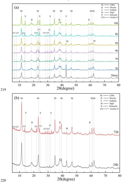
Fig. 3. XRD patterns of solid products after different reaction times (a)MMS-1 (6:1:2-30L-6M-80℃), (b)MMS-4(6:1:2-30L-6M-55℃).
