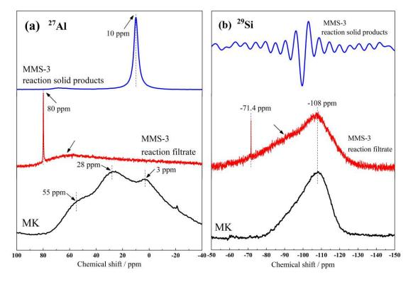
Fig. 10. (a) <sup>27</sup>Al and (b) <sup>29</sup>Si MAS-NMR spectra for the raw material MK, reaction filtrate and solid products of sample MMS-3 (6:2:1-60L-6M-80°C).
