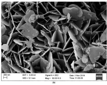
Fig. 8. SEM images of MMS-3(6:1:2-60L-6M-80°C): (a) lower magnification, (b) higher magnification on the area highlighted with a white square frame in (a).
