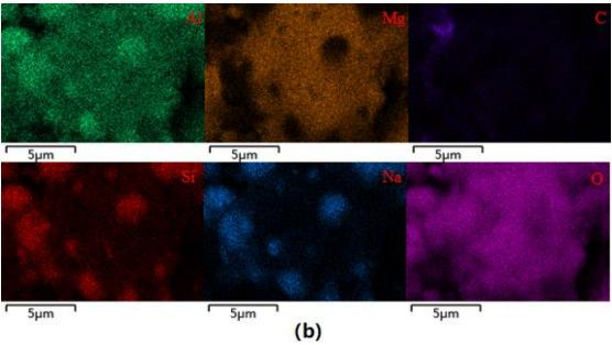
Fig. 7. (a) SEM image and EDS data at Point 1(b) EDS mapping of MMS-1 (6:1:2-30L-6M-80°C).
