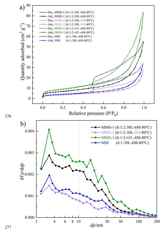
Fig. 6. BET test results of solid products synthesized from MgO and MK. (a)  $N_2$  physisorption isotherm and (b) pore size distribution calculated by BJH method.
