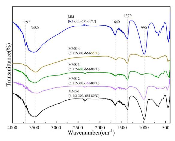
Fig. 4. FTIR spectra of solid products synthesized from MgO and MK.
