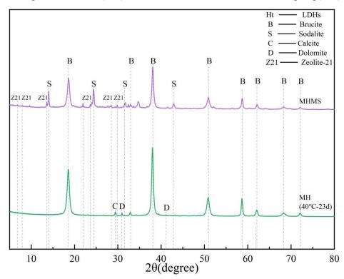
Fig. 9. XRD patterns of the solid product (MHMS) synthesized from hydrated MgO (MH) and MK under the same conditions as MMS-1. (Hydrated MgO:MK:Na<sub>2</sub>CO<sub>3</sub>=6:1:2, liquid/solid ratio=30:1, 6 mol/L NaOH solution, T=80°C, t=24h).
