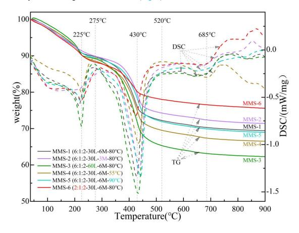
Fig. 5. TG/DSC curves of solid products synthesized from MgO and MK.
