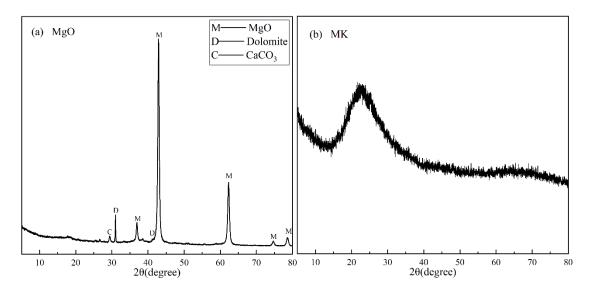
Fig. 1. XRD patterns of the raw materials (a) MgO (PDF#79-0612)
