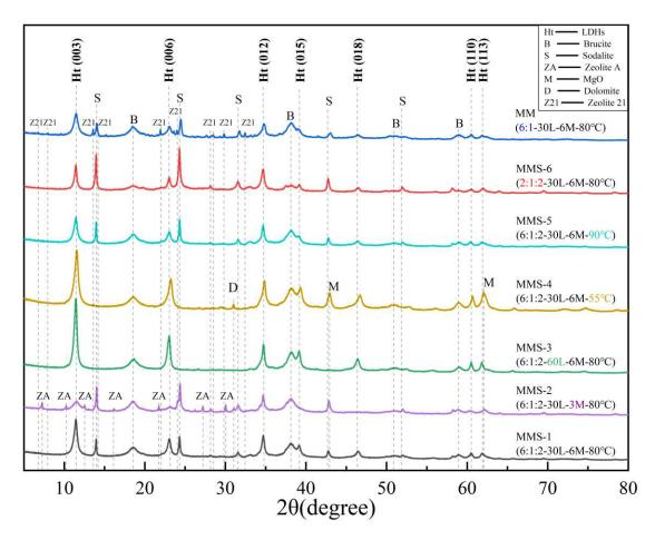
Fig. 2. XRD patterns of solid products synthesized from MgO and MK after 24h of reaction.
