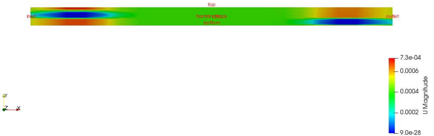
Figure A-0-25 Heterogeneous Darcy-scale simulation example with two low hydraulic conductivity zones in the waste mass (velocity field of leachate shown, flowing in from the left).
