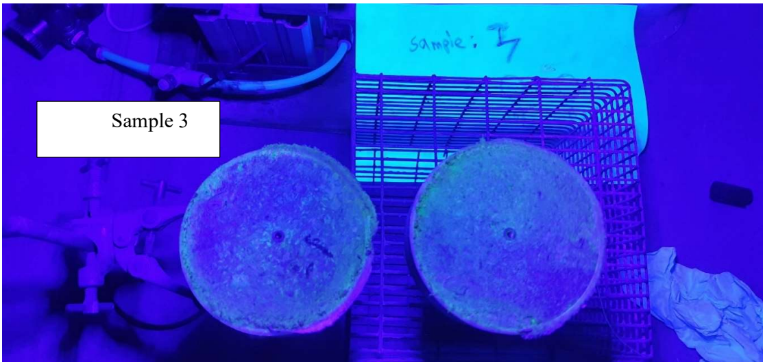
Figure A-0-21 Heterogeneous lab-scale landfills. Experimental conditions: NOFLOW+NEWS12g+SAND600g+METHANO+M9.
