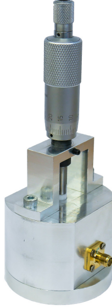
Fig. 7. C-band LODR fixture operating in the TE_{01\delta} mode around 7.58 GHz with dielectric at the base (i.e. x = 0 mm). Coupling is achieved inductively by two loop-terminated SMA ports.
