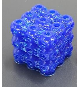
Figure 3.17. A NinjaFlex TPU SP structure pad, additively manufactured for mechanical testing validation. Stringing is visually apparent, where excess material oozes from the nozzle as it paths between printing regions.
