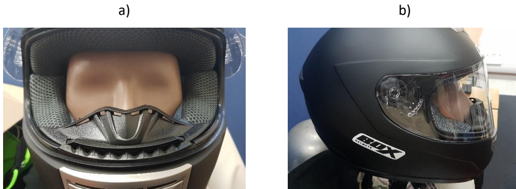
Figure 3.25. The fit of the BOX BX-1 helmet on a representative headform, a) front view, b) side view
