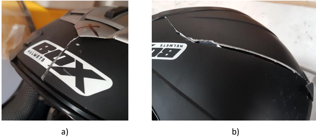
Figure A.15. Photos of the crack which propagated in the SP filled helmet's shell, after multi-impacts at, a) front, b) rear
