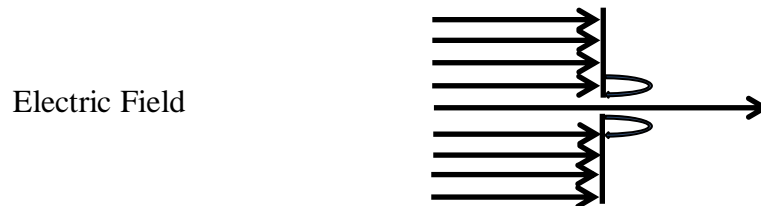
Fig. 2.13: Coupling of an electric field through an aperture – Normal to plane of aperture
