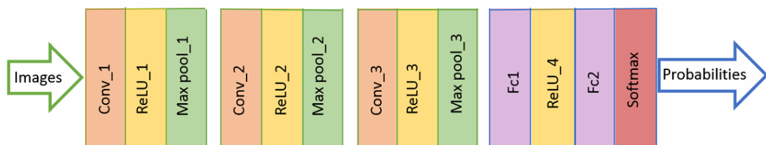
Figure 4-1: Schematic architectures of the CIFAR classification network.
