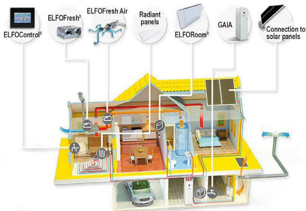
Figure 5.4 Components for Clivet's ELFOSystem GAIA for 'Class A' single-family houses (Clivet 2011)
