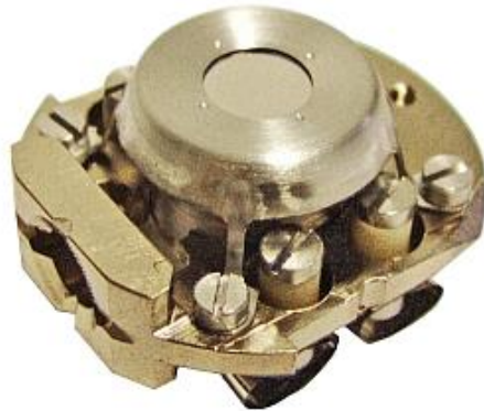
Figure 2. Picture of a conventional LEEM sample holder. (Figure adapted from [10] with permission from publisher).
