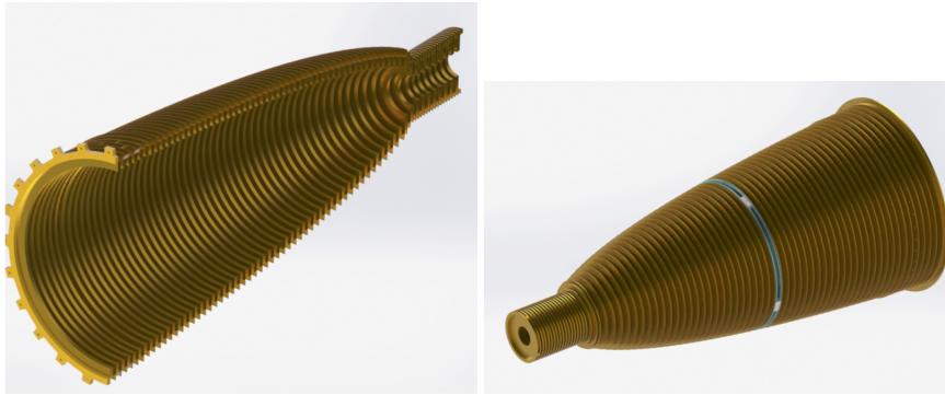
Fig. 3 Left: horn longitudinal cut through ring diameters. Right: Opposite view, with a suspension point in a machined ring in the middle of the horn (green ring).
