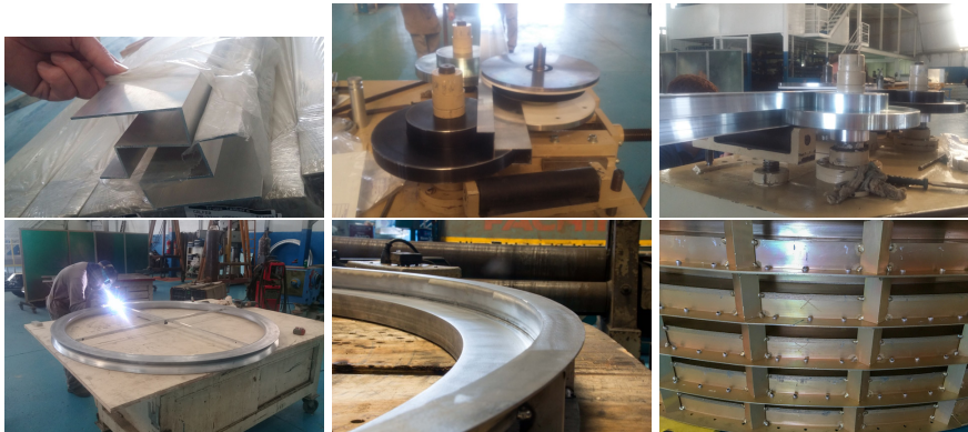
Fig. 4 The horn construction process. Starting from chair-shaped profiles bent out of a single sheet of aluminum (top-left), these profiles are then bent into rings. Top-middle: View of the 3 rollers used for conformation. Top-right: Side view of the fitting of the profile onto the rollers. Before being welded together to produce a complete ring (bottom-left) and any deviations smoothed out (bottom-middle). They are then stacked and riveted to each other (bottom-right) to form the complete horn
