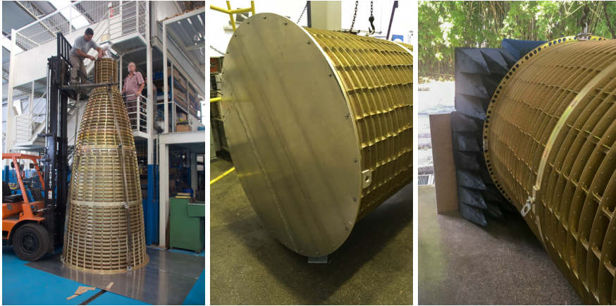
Fig. 6 Left: Initial horn testing at Calfer. Middle: Testing the horn at INPE with a aluminum plate covering the horn aperture. Right: At INPE with Eccosorb covering the horn aperture
