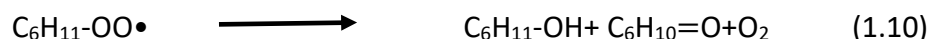
Scheme 1.2: Reaction Mechanism for the production of cyclohexanol and cyclohexanone from cyclohexyl hydroperoxide
