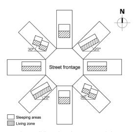
Fig. 1 Building orientation recommendations
