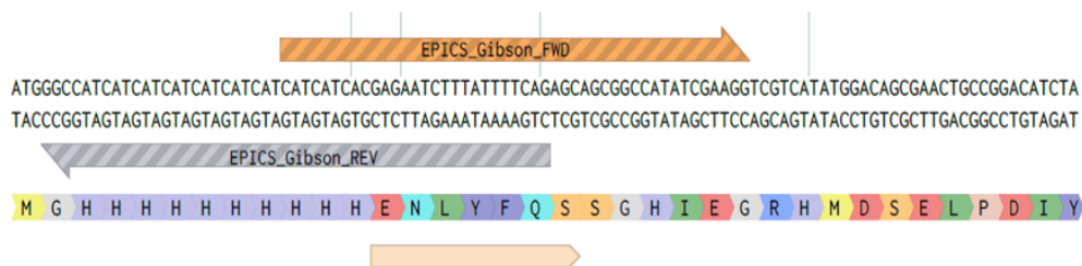
Figure 48. Section of the DNA sequence of GdolS highlighting designed primers for the TEV cleavage site insertion via Gibson assembly. [210]
