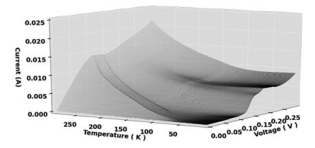
Forward bias I(V) characteristic of a symmetrical TBRTS. The temperature dependent resonant current peak can be seen emerging at  $\sim 60K$  and continues to increase in magnitude up to 293K.
