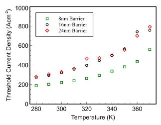
Figure 1: Threshold current density against temperature for a 2mm cavity length lasers, for each barrier width.
