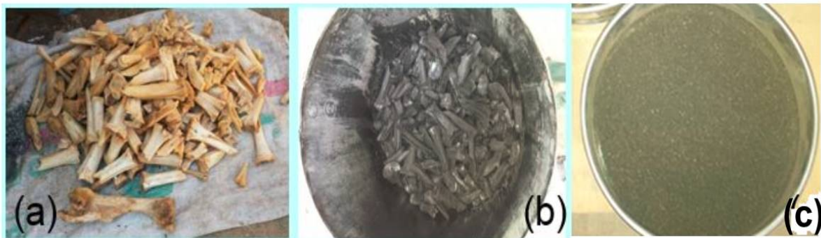
Figure 4: Dried washed, tendon and flesh- free cow bones (a). Dark coloured cow bones after charring in the furnace at 530°C for 30 minutes (b). Sieved faction (0.2-0.8mm) of powdered charred bones (c)
