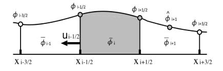
Figure 3.2: Schematic figures of the CIP-CSL3U scheme.  $u_{i-1/2} < 0$  is assumed. The moments which are indicated by grey colour are used as constraints to construct interpolation function  $\Phi_i^{CSL3U}(x)$ .
