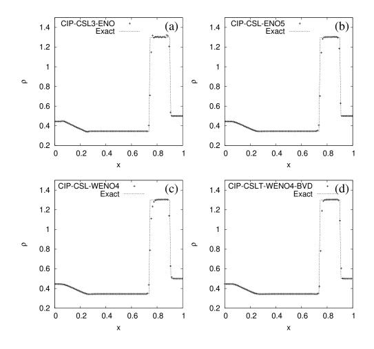
Figure 5.2: Numerical results of Lax's shock tube problem at t=0.16 and N=100. (a) CIP-CSL3-ENO, (b) CIP-CSL-ENO5, (c) CIP-CSL-WENO4, (d) CIP-CSLT-WENO4-BVD.
