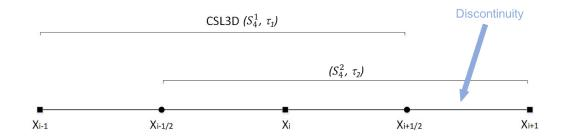
Figure 4.5: Reconstruction stencils for the CIP-CSL-ENO5 scheme. The discontinuity exists in the region of upwind-side between  $x_{i+1/2}$  and  $x_{i+1}$ , CSL3D is used as the reconstruction scheme.
