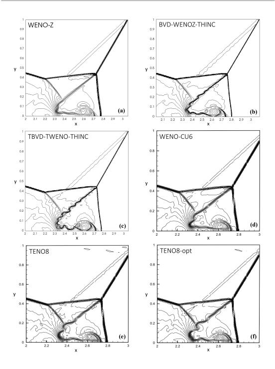
Figure 6.17: Zoomed-in view of double-Mach reflection test with a qualitative comparison: density contours by (a) WENO-Z, (b) BVD-WENOZ-THINC, (c) TBVD-TWENO-THINC, (d) WENO-CU6, (e) TENO8 and (f) TENO8-opt at t = 0.2, with a  $512 \times 128$  mesh. This figure is drawn with density contours between 1.887 and 20.9.
