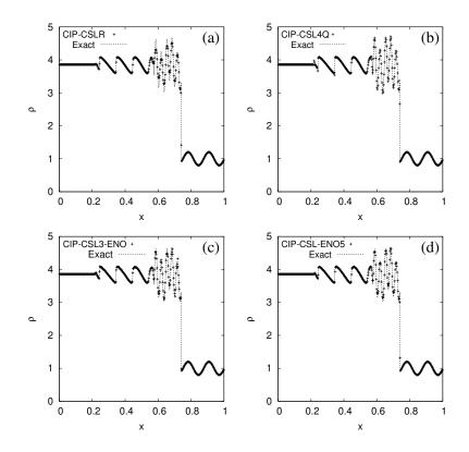
Figure 4.12: Numerical results of shock-turbulence interaction problem at time t=0.18. N=400 and CFL=0.2 are used. (a) CIP-CSLR, (b) CIP-CSL4Q, (c) CIP-CSL3-ENO, (d) CIP-CSL-ENO5.
