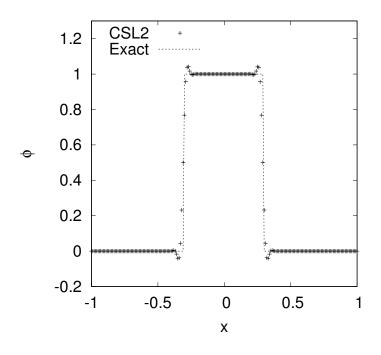
Figure 2.5: The simulation of the advection of a square wave by the CSL2 scheme on a 100-cell mesh.
