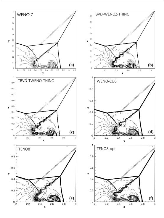
Figure 6.18: Zoomed-in view of double-Mach reflection test with a qualitative comparison: density contours by (a) WENO-Z, (b) BVD-WENOZ-THINC, (c) TBVD-TWENO-THINC, (d) WENO-CU6, (e) TENO8 and (f) TENO8-opt at t = 0.2, with a  $1024 \times 256$  mesh. This figure is drawn with density contours between 1.887 and 20.9.
