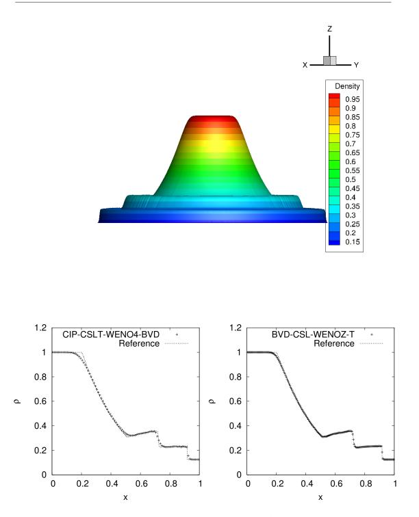
Figure 5.4: 2D circular explosion results of the CIP-CSLT-WENO4-BVD scheme at t=0.25. The density profile, side view (top) and the density profile along the cross-section of x = y with  $200 \times 200$  meshes (bottom left) and  $400 \times 400$  meshes (bottom right).
