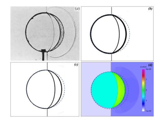
Figure 7.4: Results for a planar Mach 1.22 shock wave in air interacting with a circular R22 gas bubble at  $t = 55 \ \mu s$ . (a) experiment, (b) VOF, (c) VOF with interface-sharpening, and (d) TBVD-TWENO-THINC.
