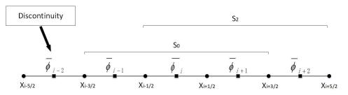
Figure 6.2: Discontinuity exists in sub-stencil  $S_1$ , while adjacent sub-stencils  $S_0$  and  $S_2$  are smooth.
