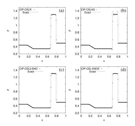
Figure 4.11: Numerical results of Lax's shock tube problem at t=0.12. N=200 and CFL=0.2 are used. (a) CIP-CSLR, (b) CIP-CSL4Q, (c) CIP-CSL3-ENO, (d) CIP-CSL-ENO5.
