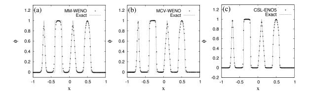
Figure 4.10: A comparison of numerical results by the multi-moment WENO scheme, the MCV-WENO scheme, and the CIP-CSL-ENO5 scheme in complex wave propagation test at t=2 (1 period: 500 time steps). N=200 and CFL=0.4 are used.
