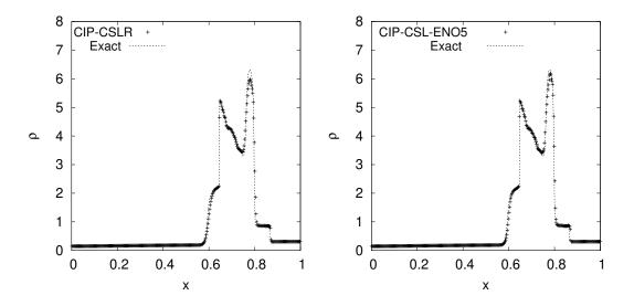
Figure 4.14: Numerical results of two interacting blast waves problem at t=0.038. N=400. CIP-CSLR (left) and CIP-CSL-ENO5 (right).
