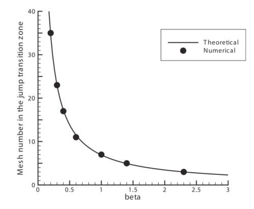
Figure 6.4: The relationship between the parameter  $\beta^T$  and the mesh number in the jump transition zone. [2].
