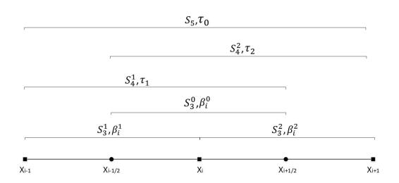
Figure 4.2: Sketch of the reconstruction stencils of the CIP-CSL-ENO5 scheme.
