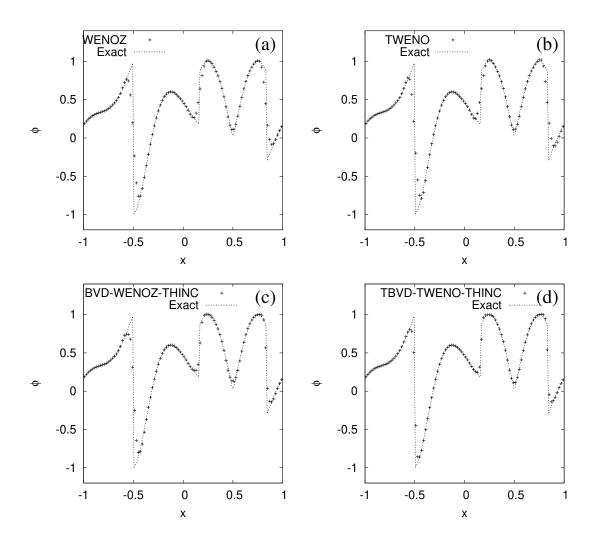
Figure 6.8: Numerical results of capturing the extrema of the various smoothness test at t=2. N=100 and CFL=0.4 are used. (a) WENO-Z, (b) TWENO, (c) BVD-WENOZ-THINC, (d) TBVD-TWENO-THINC.
