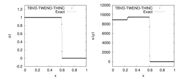
Figure 7.2: Numerical results of the two-material impact test. N=200,  $t = 85 \mu s$ . left: volume fraction ( $\alpha 1$ ), right: mass fraction ( $\alpha 1 \rho 1$ ).
