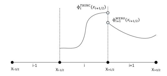
Figure 2.6: Illustration of one possible situation corresponding to  $|\Phi_i^{THINC}(x_{i+1/2}) - \Phi_{i+1}^{WENO}(x_{i+1/2})|$  when calculating boundary variation at  $x_{i+1/2}$ .
