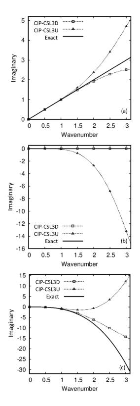
Figure 3.3: Spatial derivatives of the CIP-CSL3D and CIP-CSL3U schemes at a cell boundary  $x_{i-1/2}$ . The results of imaginary parts of (a) first derivatives, (b) second derivatives, (c) third derivatives.
