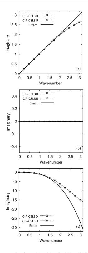
Figure 3.5: Spatial derivatives of the CIP-CSL3D and CIP-CSL3U schemes at the cell centre  $x_i$ . The results of imaginary parts of (a) first derivatives, (b) second derivatives, (c) third derivatives.
