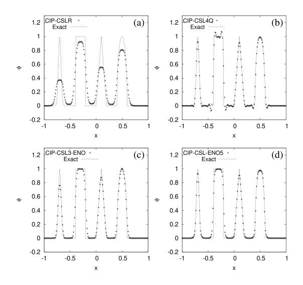
Figure 4.8: Numerical results of complex wave propagation test at time t=100 (50 periods). N=200 and CFL=0.4 are used. (a) CIP-CSLR, (b) CIP-CSL4Q, (c) CIP-CSL3-ENO, (d) CIP-CSL-ENO5.
