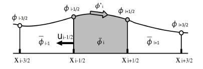
Figure 2.3: Schematic figures of the CIP-CSL3 scheme. The moments which are indicated by grey colour are used as constraints to construct interpolation function  $\Phi_i^{CSL3}(x)$ . The wave propagation speed  $u_{i-1/2} < 0$  is assumed.
