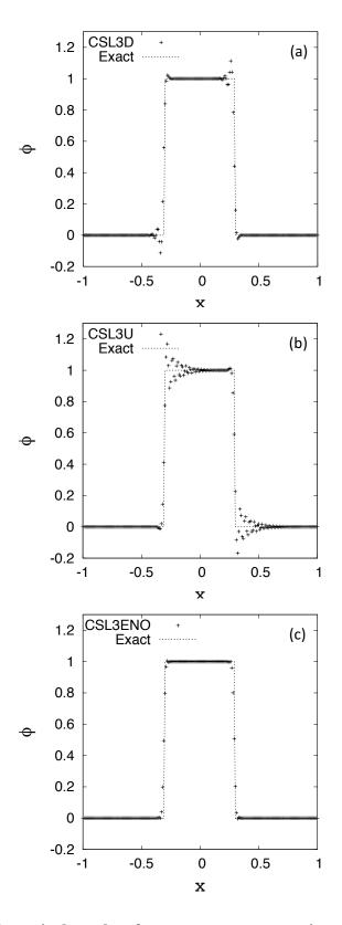
Figure 3.6: Numerical results of square wave propagation test at t=16 (8,000 time steps). N=200 and CFL=0.2 are used. (a) CIP-CSL3D, (b) CIP-CSL3U, (c) CIP-CSL3-ENO.
