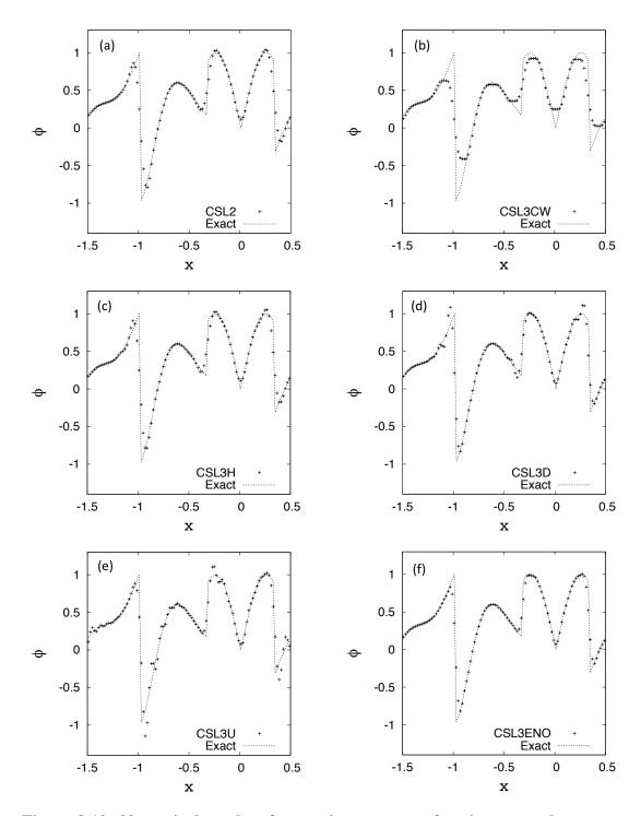
Figure 3.10: Numerical results of capturing extrema of various smoothness test at t=8. N=100 and CFL=0.4 are used. (a) CIP-CSL2, (b) CIP-CSL3CW, (c) CIP-CSL3H, (d) CIP-CSL3D, (e) CIP-CSL3U, (f) CIP-CSL3-ENO.
