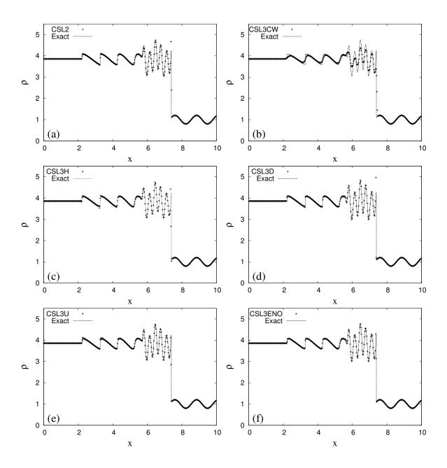
Figure 3.15: Numerical results of shock-turbulence interaction problem at t=1.8 (CFL=0.2 and N=400). (a) CIP-CSL2, (b) CIP-CSL3CW, (c) CIP-CSL3H, (d) CIP-CSL3D, (e) CIP-CSL3U, (f) CIP-CSL3-ENO.
