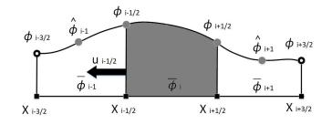
Figure 4.1: Schematic figure of the CIP-CSL4Q scheme.  $u_{i-1/2} < 0$  is assumed. The moments which are indicated by grey colour are used as constraints to construct the interpolation function  $\Phi_i^{CSL4Q}(x)$ .
