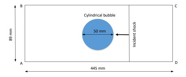
Figure 7.3: A schematic of the computational domain
