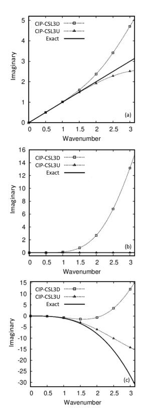
Figure 3.4: Spatial derivatives of the CIP-CSL3D and CIP-CSL3U schemes at a cell boundary  $x_{i+1/2}$ . The results of imaginary parts of (a) first derivatives, (b) second derivatives, (c) third derivatives.
