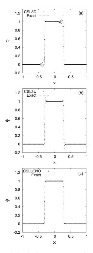
Figure 3.7: Numerical results of square wave propagation test at t=16 (2,000 time steps). N=200 and CFL=0.8 are used. (a) CIP-CSL3D, (b) CIP-CSL3U, (c) CIP-CSL3-ENO.
