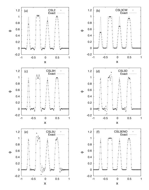
Figure 3.8: Numerical results of complex wave propagation test at t=16 (4,000 time steps, 8 period). CFL=0.4 and N=200 are used. (a) CIP-CSL2, (b) CIP-CSL3CW, (c) CIP-CSL3H, (d) CIP-CSL3D, (e) CIP-CSL3U, (f) CIP-CSL3-ENO.
