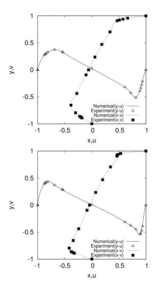
Figure 4.15: The horizontal velocity component u along the x = 0.5 axis and the vertical velocity component v along the y = 0.5 axis. Displayed are the results of the CIP-CSL-ENO5 scheme on  $100 \times 100$  meshes with the Reynolds number being 1000 (top) and 3200 (bottom) respectively.
