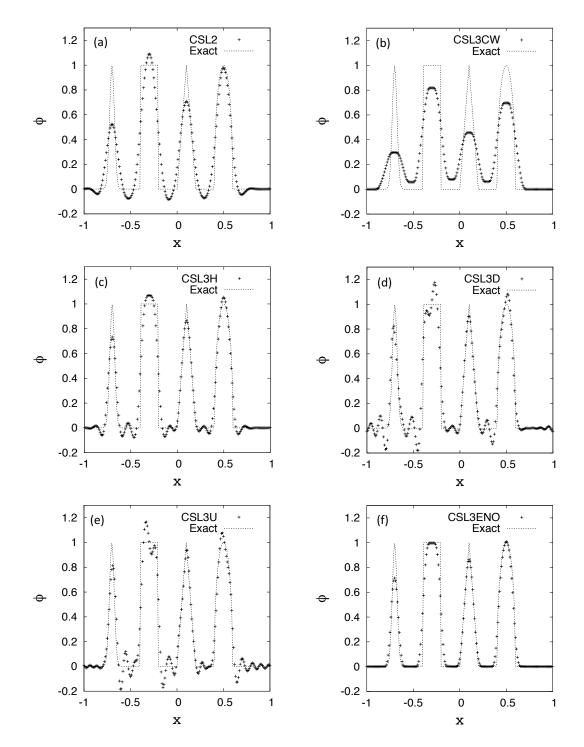
Figure 3.9: Numerical results of complex wave propagation test at t=160 (40,000 time steps, 80 period). CFL=0.4 and N=200 are used. (a) CIP-CSL2, (b) CIP-CSL3CW, (c) CIP-CSL3H, (d) CIP-CSL3D, (e) CIP-CSL3U, (f) CIP-CSL3-ENO.
