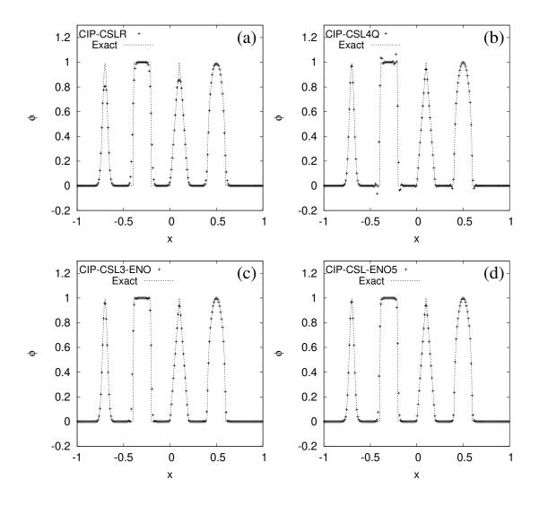
Figure 4.7: Numerical results of complex wave propagation test at time t=2 (1 period). N=200 and CFL=0.4 are used. (a) CIP-CSLR, (b) CIP-CSL4Q, (c) CIP-CSL3-ENO, (d) CIP-CSL-ENO5.
