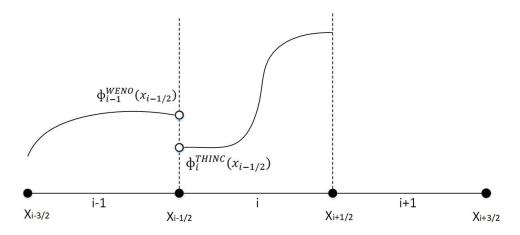
Figure 2.7: Illustration of one possible situation corresponding to  $|\Phi_{i-1}^{WENO}(x_{i-1/2}) - \Phi_i^{THINC}(x_{i-1/2})|$  when calculating boundary variation at  $x_{i-1/2}$ .
