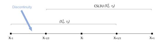
Figure 4.4: Reconstruction stencils for the CIP-CSL-ENO5 scheme. The discontinuity exists in the region of downwind-side between  $x_{i-1}$  and  $x_{i-1/2}$ , CSL3U is used as the reconstruction scheme.
