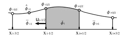
Figure 3.1: Schematic figures of the CIP-CSL3D scheme.  $u_{i-1/2} < 0$  is assumed. The moments which are indicated by grey colour are used as constraints to construct interpolation function  $\Phi_i^{CSL3D}(x)$ .
