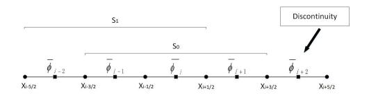
Figure 6.3: Discontinuity exists in sub-stencil  $S_2$ , while adjacent sub-stencils  $S_0$  and  $S_1$  are smooth.
