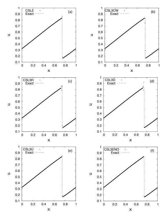
Figure 3.11: Numerical results of Burgers' equation at t=1. N=200 and CFL=0.2 are used. (a) CIP-CSL2, (b) CIP-CSL3CW, (c) CIP-CSL3H, (d) CIP-CSL3D, (e) CIP-CSL3U, (f) CIP-CSL3-ENO.
