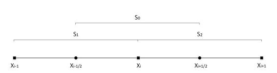
Figure 2.4: Reconstruction stencils for the weighted essentially non-oscillatory limiter.
