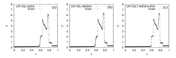
Figure 5.3: Numerical results of two interacting blast waves problem at t=0.038 and N=400. (a) CIP-CSL-ENO5, (b) CIP-CSL-WENO4, (c) CIP-CSLT-WENO4-BVD.
