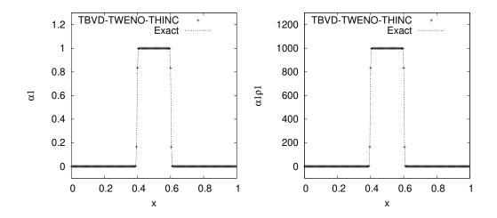
Figure 7.1: Numerical results of a passive advection of a square liquid column. N=200, t = 10 ms. Left: volume fraction ( $\alpha 1$ ), right: mass fraction ( $\alpha 1\rho 1$ ).
