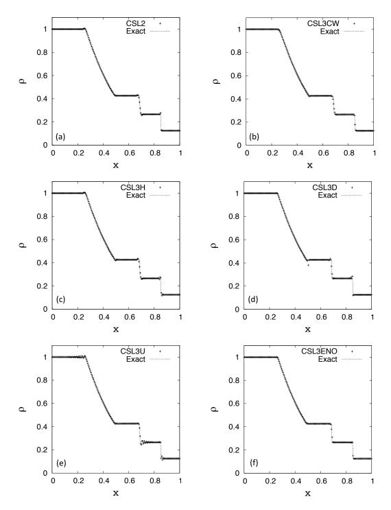
Figure 3.13: Numerical results of Sod's shock tube problem at t = 0.2 (N=200 and CFL=0.2). (a) CIP-CSL2, (b) CIP-CSL3CW, (c) CIP-CSL3H, (d) CIP-CSL3D, (e) CIP-CSL3U, (f) CIP-CSL3-ENO.
