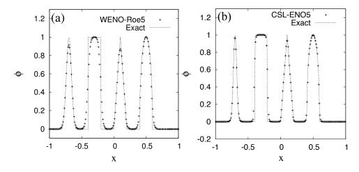
Figure 4.9: A comparison of numerical results by the WENO-Roe5 scheme [1] and the CIP-CSL-ENO5 scheme in complex wave propagation test at t=8 (4 periods: 2,000 time steps). N=200 and CFL=0.4 are used.
