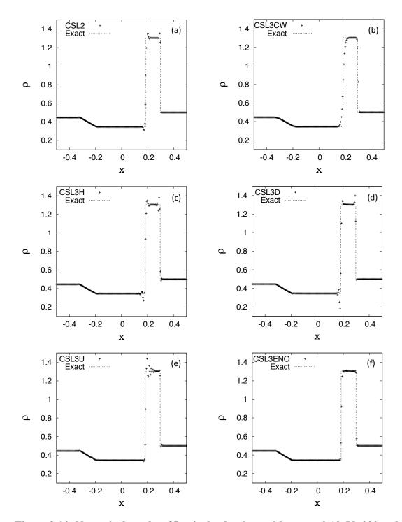
Figure 3.14: Numerical results of Lax's shock tube problem at t=0.12 (N=200 and CFL=0.2). (a) CIP-CSL2, (b) CIP-CSL3CW, (c) CIP-CSL3H, (d) CIP-CSL3D, (e) CIP-CSL3U, (f) CIP-CSL3-ENO.
