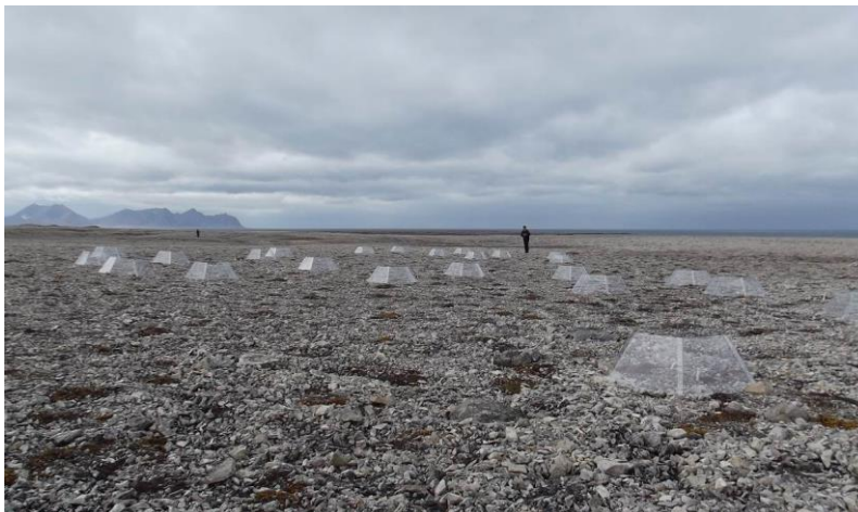
Figure 2.6 The High Arctic soil warming experiment. Forty-eight plots were established over soil polygons in September 2014. Open top chambers provided a warming treatment, whilst deionised water was applied to simulate increased precipitation, resulting in four treatment types, each replicated 12 times over three blocks.
