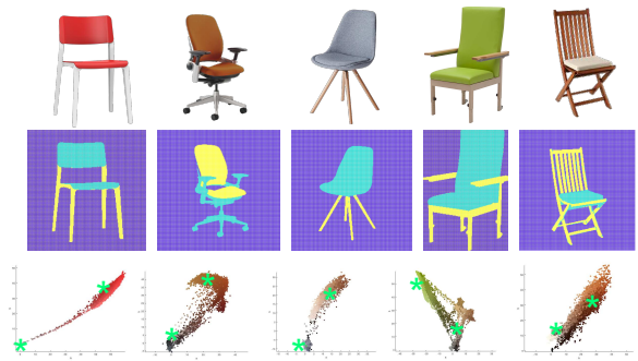
Fig. 3: Image segmentations by k -means. Top row: 5 original retrieved images after pruning. Middle row: the corresponding segmentation results (colomap indicating different segmented regions) by setting k = 2 . Bottom row: the Lab color space (L component for lightness is discarded) of all pixels along with 2 cluster centroids marked as green stars.
