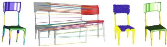
Fig. 8: Matching process. From left to right: the pre-segmented 3D model, the dense correspondence between rendered view of model and 2D image, the label-transferred samples on mesh, the labeled 3D patches by majority voting.
