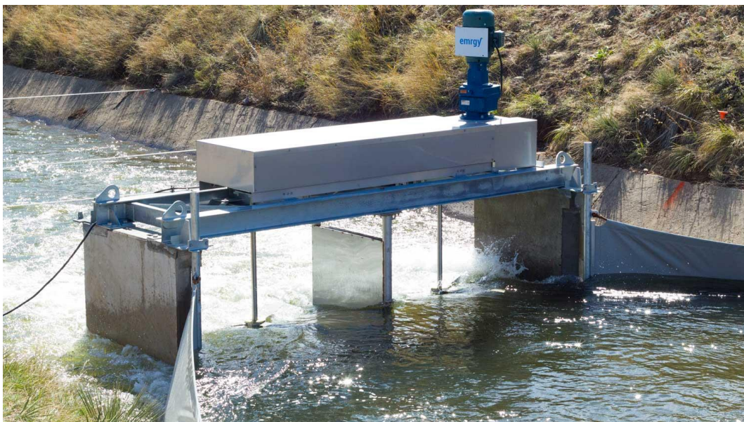
Figure 1.3. The hydrokinetic energy conversion system developed by Emrgy [7].
