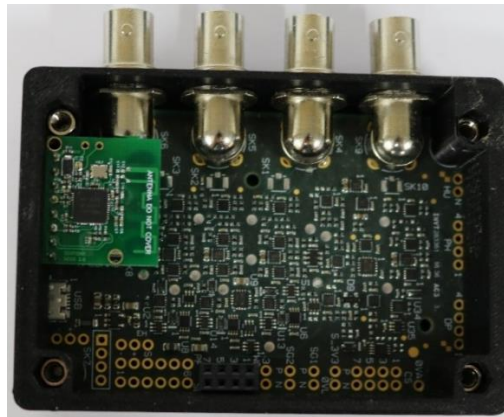
Figure 109 – Mk 2 node within 3D printed case
