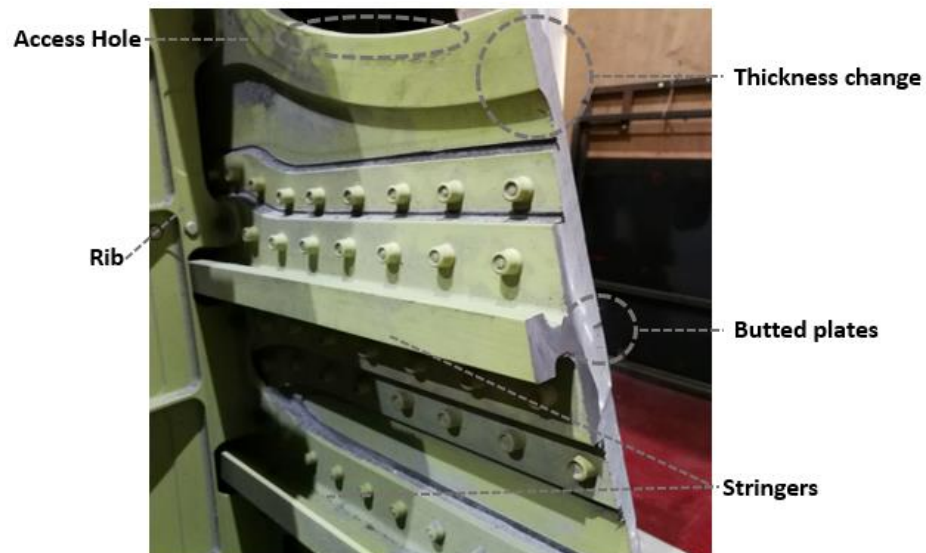
Figure 7 – Internal structure of an aluminium A320 wing showing a stringer and rib bonded and riveted. Also shown are a thickness change, an edge due to access hole and where two plates are butted together and reinforced by the stiffeners
