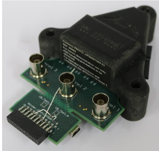
Figure 99 – Mk 1 node in 3D printed casing
