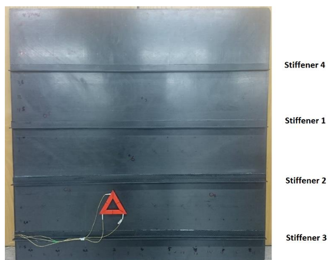
Figure 43 – Composite panel B with four stiffeners bonded
