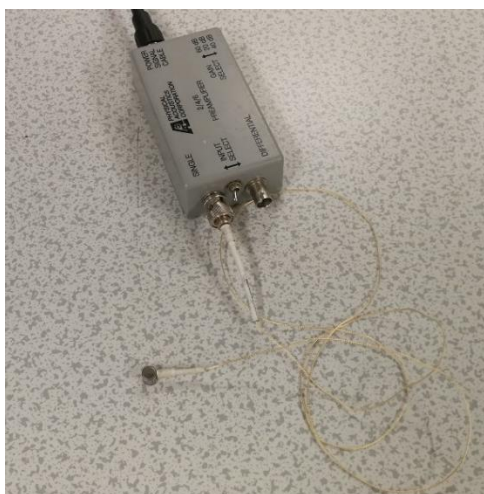
Figure 26 - Pre-amplifier and Nano-30 AE sensor
