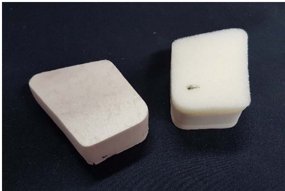
Fig. 1. The two foam parts removed from the American football helmet, one showing the comfort foam removed (left) and the other still intact (right)
