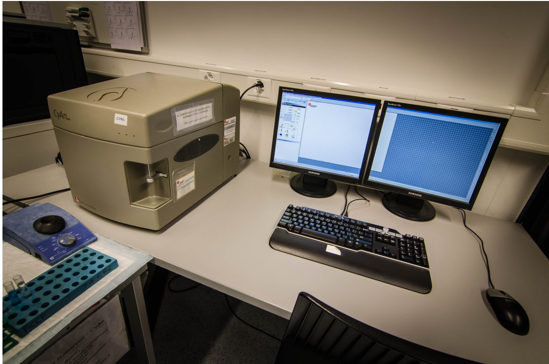
Figure 23: CyAn flow cytometer. (Beckman Coulter), with Summit software. Capable of 11 simultaneous parameters (forward and side scatter with 7-9 colours and simultaneous width, peak, area and log on each).
