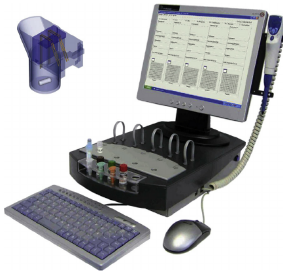
Figure 22: Multiplate platelet analyser. (Roche diagnostics). A five channel impedance analyzer, (inset) disposable cuvettes with electrodes and stir bar.
