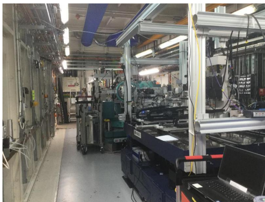
Figure 8.1 The synchrotron experimental hutch of beamline B16 in Diamond Light Source (Didcot, Oxfordshire), where all the XBI experiments reported in this thesis were carried out. The green equipment in the middle of the hutch is the Huber diffractometer.
