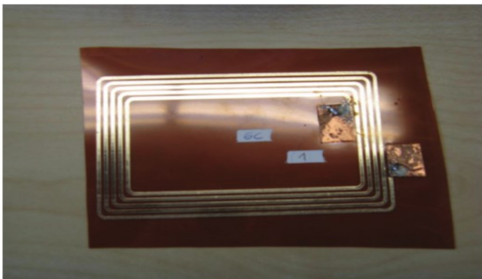
Figure 3.6 – Printed antenna prototype. [20]
