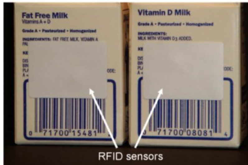
Figure 3.8 – Milk cartons with RFID sensors attached. [32]
