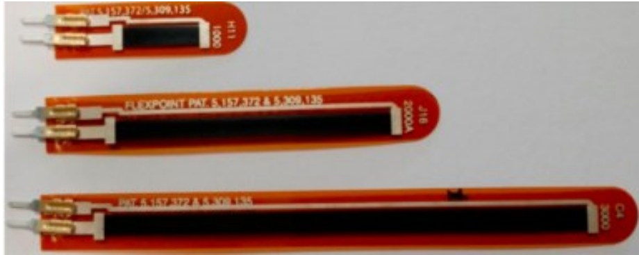
Figure 3.23 – Examples of resistive flex sensors, by Flexpoint Inc. [138]
