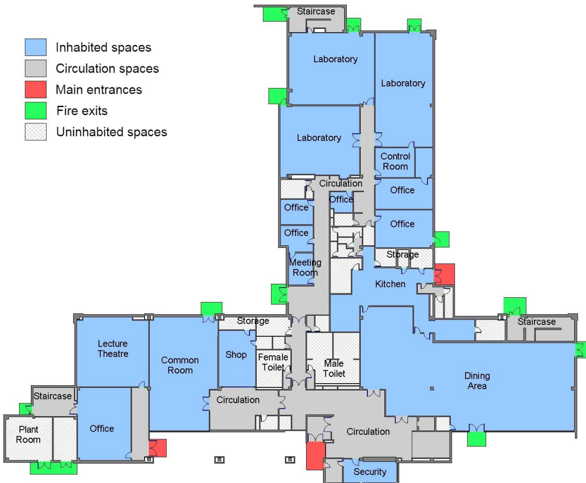
Figure 7-3. Case study building layout, ground floor
