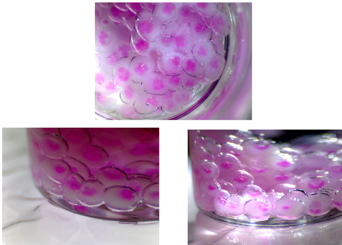
Figure 4.2 Beaker (5 mL) displaying a 3-dimensional network of adhered eDIBs in oil, forming 3D proto-tissues.
