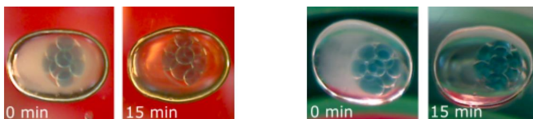
Figure 3.13 Photographs demonstrating how the alginate shell of an eDIB becomes transparent over a period of approximately 15 minutes. This occurs as acetic acid from the carrier oil phase partitions into the alginate phase, which contains suspended calcium carbonate particles that confer an initial opacity to the phase. The lowering of pH caused by the partitioning process causes these particles to be dissolved, resulting in transparency of the eDIB shell. These eDIBs have been output into a petri dish and are submerged in mineral oil containing 0.5 % v/v acetic acid.
