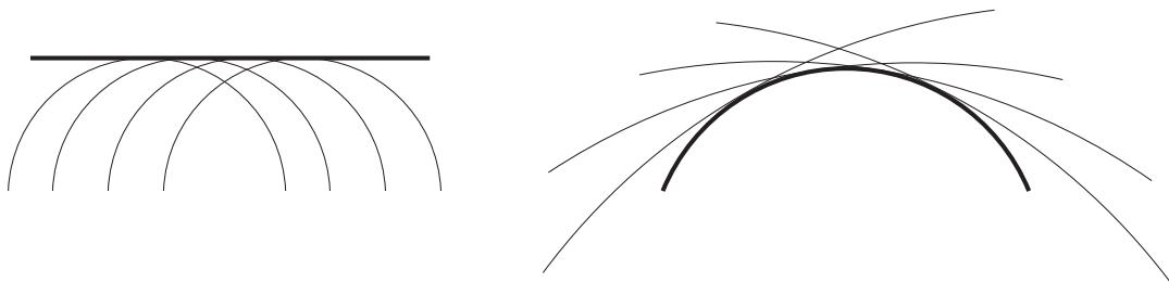
Figure 6.8: Schematic diagrams for the formation of the front and back parts of the Mach envelope (left and right respectively). In each case the thin curves are the wavefronts and the thick curve is their envelope.
