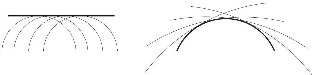
Figure 3.26: Schematic diagrams for the formation of the incident and reflected parts of the Mach envelope (left and right respectively). In each case the thin curves are the wavefronts and the thick curve is their envelope.
