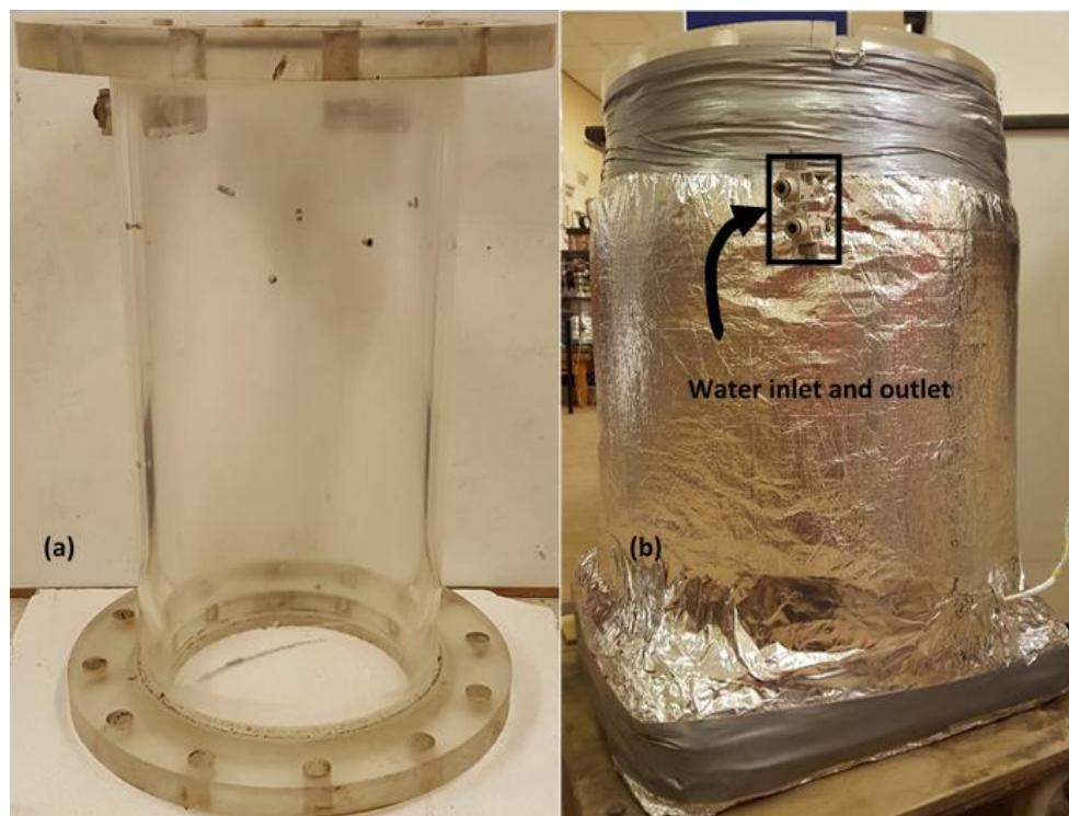
Figure (5.2) Acrylic tube before and after applying Rockwool insulation
