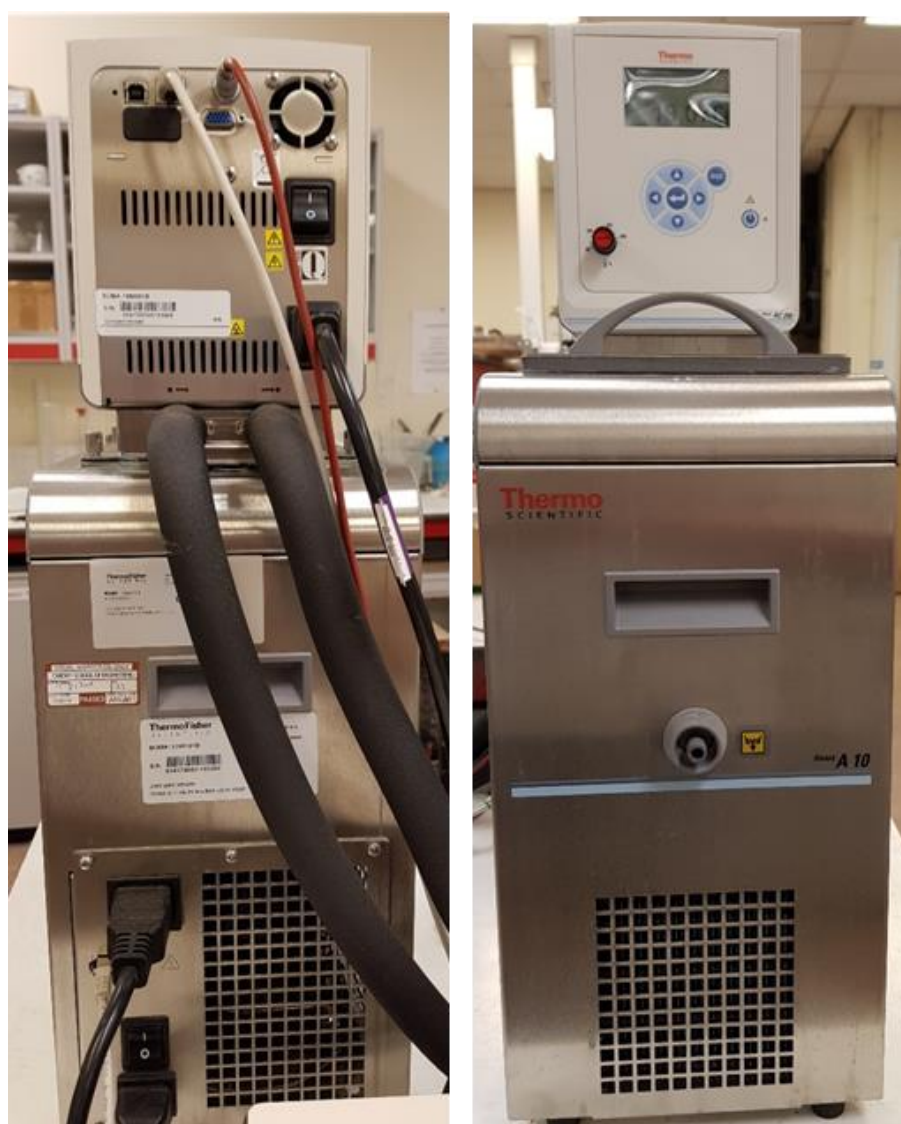
Figure (5.3) Front and back face of the circulator
