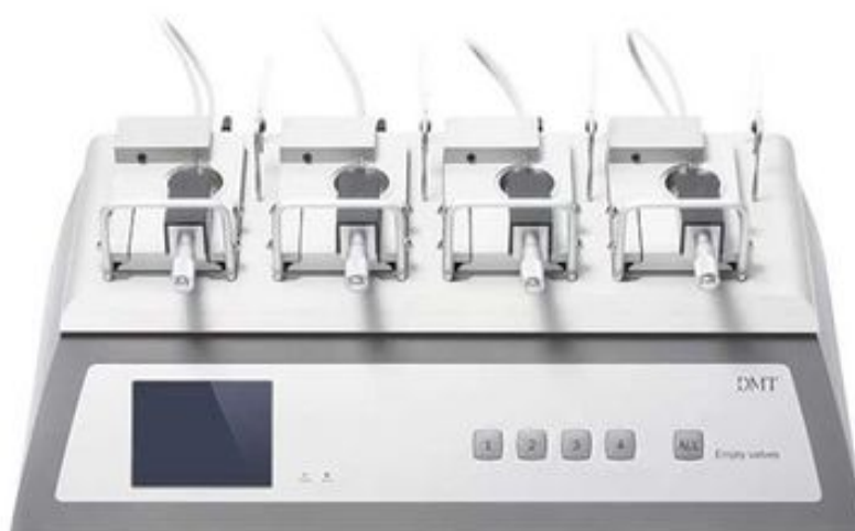
Figure 2.4: Wire myograph with four chambers (DMT, Aarhus, Dk).
