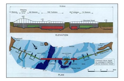
Figure 2-9 - Configuration of STPG Barrage (STPG, 1989)
