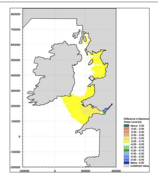
Figure 2-14 - Impact of Severn Barrage on maximum water levels (Zhou, Pan and Falconer, 2014a)
