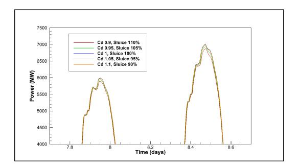
Figure 5-11 - Power generated by the barrage when varying  $C_d$  and sluice capacity
