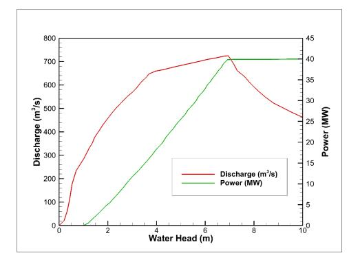
Figure 2-15- Relationship between the water head, discharge and power output (STPG, 1989)
