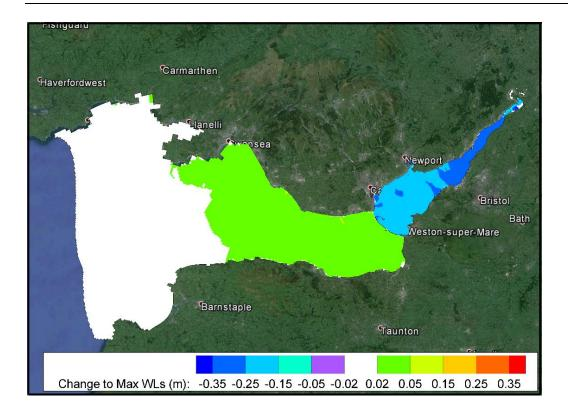
Figure 5-8 - Maximum water level changes caused by a 10% reduction in the  $C_d$
