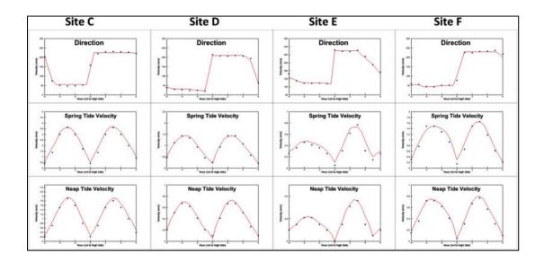
Figure 4-6 - Comparisons between observed (blue dots) and calculated (red lines) tidal stream current speeds and directions
