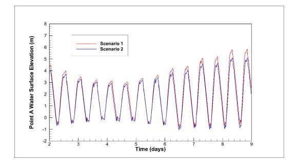
Figure 5-4 - Impact of hydraulic structure refinements on water levels at Point A
