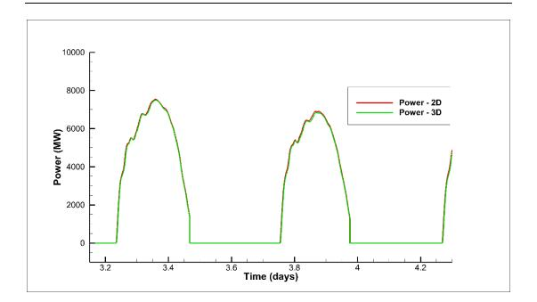
Figure 5-18 - Power output comparison for 2D and 3D STPG ebb-generating barrage simulations
