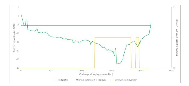
Figure 6-4 - Bed elevation profile (green), minimum water depth (blue) and potential turbine housing locations (yellow) along the Bridgwater Bay Lagoon line
