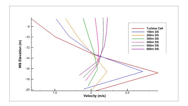
Figure 5-16 - Velocity profile through the water column 100m increments downstream of a turbine cell
