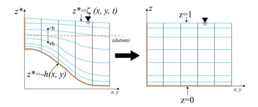
Figure 4-3 - Vertical sigma coordinate system in EFDC (Craig, 2017)
