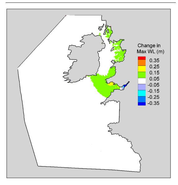
Figure 5-5 - Domain-wide maximum water level changes caused by barrage Scenario 1
