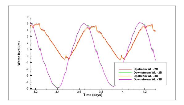
Figure 5-17 - Water levels upstream and downstream of the barrage, in 2D and 3D
