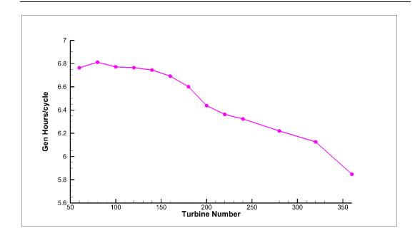
Figure 6-8 - Hours of generation per tidal cycle when varying the turbine number
