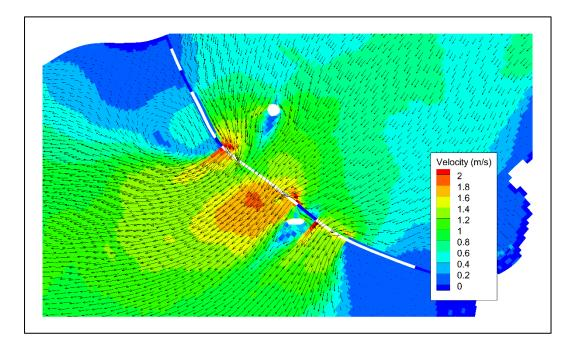
Figure 5-14 - Velocity magnitudes and vectors at mid-generating phase, pre-momentum adjustment
