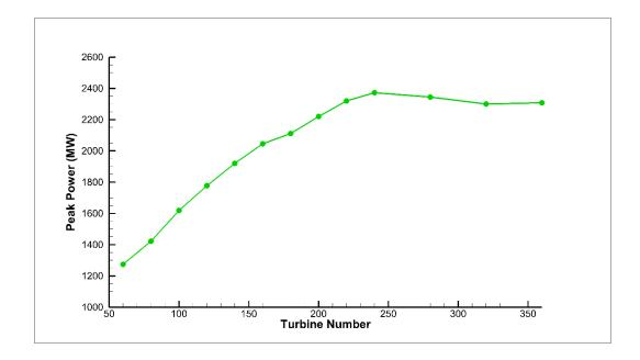
Figure 6-6 - Peak power output of the Bridgwaer Bay Lagoon when varying the turbine number
