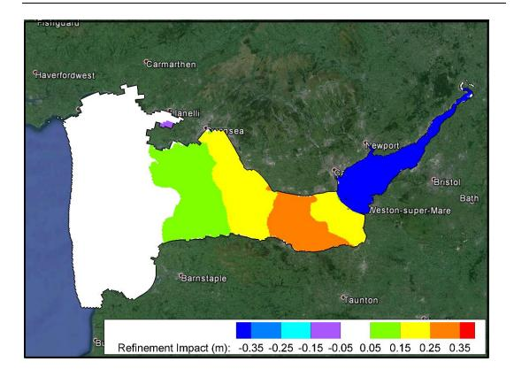
Figure 5-7 - Impact of hydraulic structure refinements on maximum water levels in the Severn Estuary and Bristol Channel
