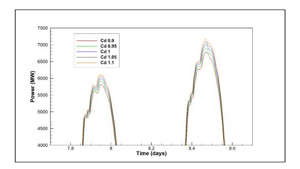
Figure 5-10 - Power generated by the barrage when varying  $C_d$  over one day
