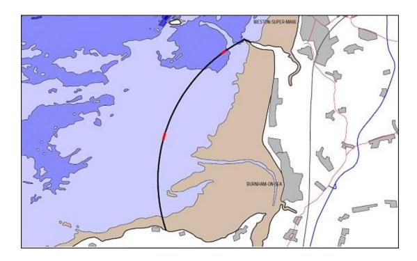
Figure 6-3 - Locations of turbines (in red) along the Bridgwater Bay Lagoon wall
