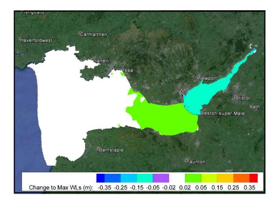
Figure 5-9 - Maximum water level changes caused by a 5% reduction in the  $C_d$  value
