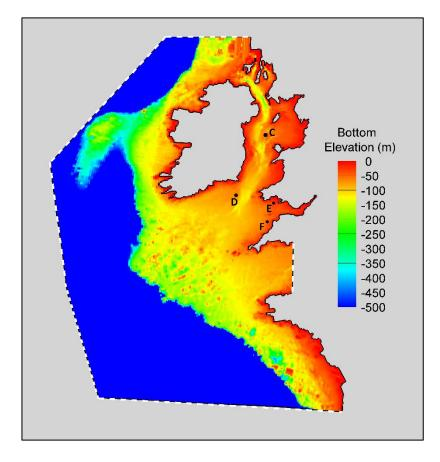
Figure 4-5 - Computational domain of the CSM, with black dots showing example validation sites and dotted lines to indicate open boundaries
