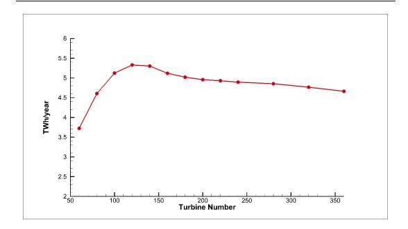
Figure 6-7- Annual energy output of Bridgwater Bay Lagoon when varying the turbine number
