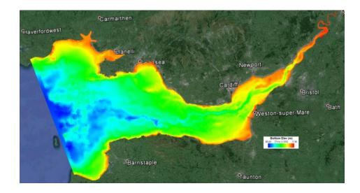
Figure 4-7 - SEM domain, showing bathymetry of the Severn Estuary and Bristol Channel
