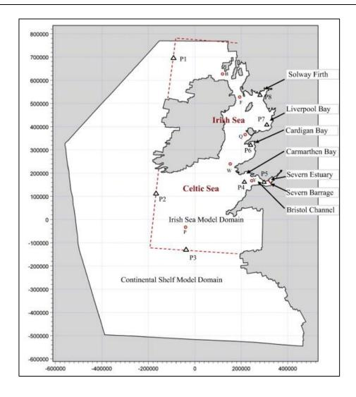
Figure 2-13 - Computational domains used to test open boundary location effect (Zhou, Pan and Falconer, 2014a)
