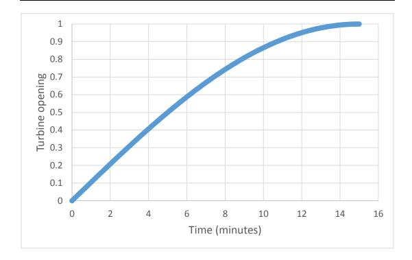
Figure 4-8 - Turbine half-sinusoidal ramp function
