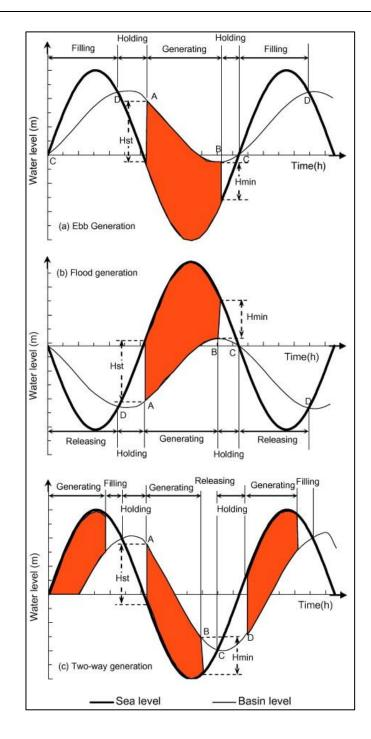
Figure 2-2 - Barrage operating modes (Xia et al., 2010b)
