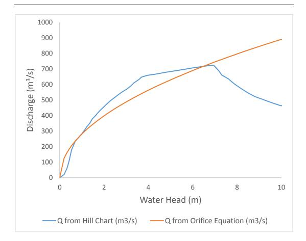
Figure 2-16 - Discharge through a turbine as calculated from the hill chart and from the orifice equation
