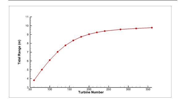
Figure 6-9 - Tidal range within the Bridgwater Bay Lagoon when varying the turbine number
