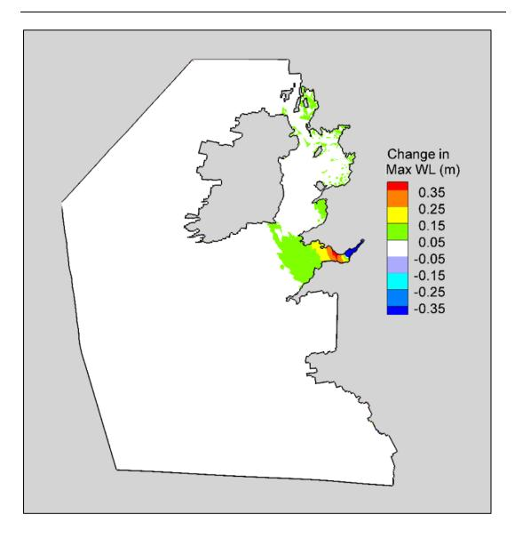
Figure 5-6 - Domain-wide maximum water level changes caused by barrage Scenario 2
