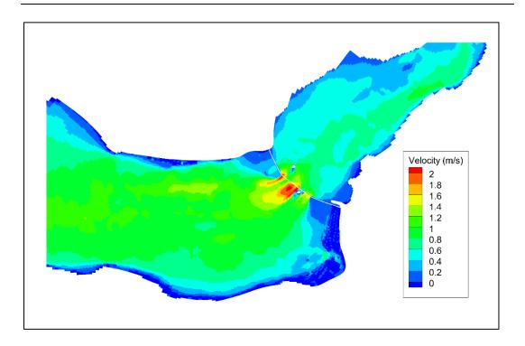
Figure 5-13 - Velocity magnitudes at mid-generating phase, post-momentum adjustment
