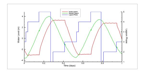
Figure 6-5 - Bridgwater Bay Lagoon operational phases
