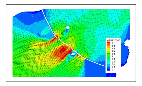
Figure 5-15 - Velocity magnitudes and vectors at mid-generating phase, post-momentum adjustment
