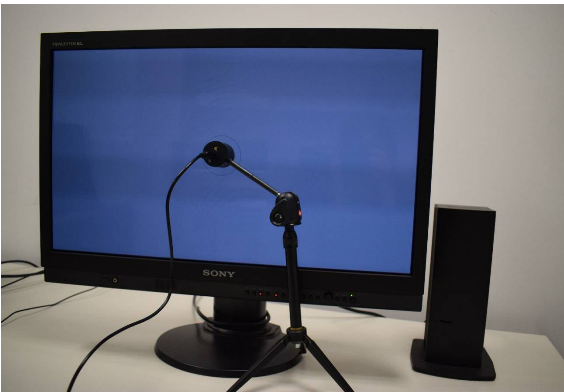
Figure 2.9 – Apparatus set-up to measure luminance output over time. The Sony PVM-A250 Trimaster EI OLED display with a (nominally) uniform background of \sim 10 \text{ cd/m}^2 . A black circle demarcates the area in which the ColorCAL II was positioned to measure the luminance output. The ColorCAL II was immobilised on a stand to ensure that all luminance output measurements were taken at the same location. The same process was also conducted with the Hewlett Packard p1230 chromatic CRT display.
