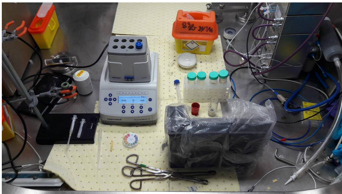
Figure 8. Experimental set-up for ^{89}\text{Zr} labelling of APTES@SPION. Care must be taken to arrange hot cell interior prior to introduction of radiation to facilitate ease of manipulation.
