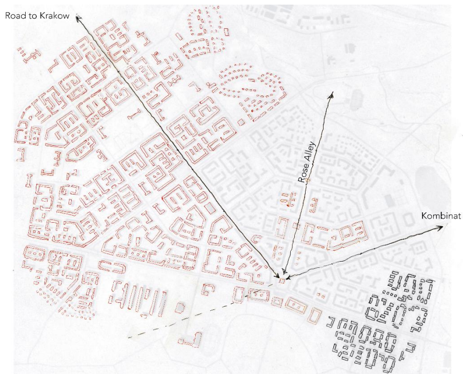
Fig. 4.46 The initial proposal for the Masterplan (Garliński 1953 81) with an overlaid sketch showing the buildings which were not erected (in red outline) and buildings that were erected according to an unassociated architectural scheme by Adamski (in black outline)
