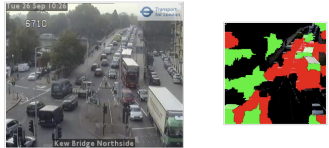
Fig. 3. Original input image (left) and saliency map (right: red regions show evidence towards ‘congested’, green regions show evidence towards ‘not congested’)
